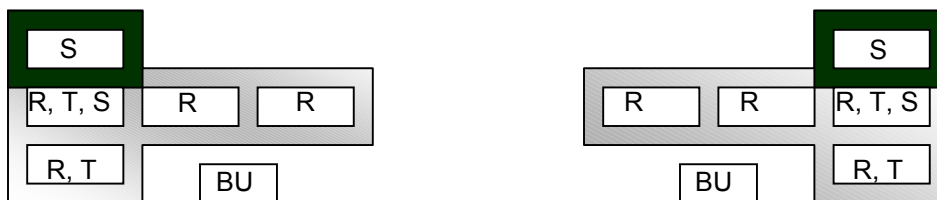
Figure 1. The proposed rear-signaling system of Projector, Cook, & Peterson (1969). In the diagram, S = Stop Lamp, R = Running Light, T = Turn signal, BU = Back-up Lights.
